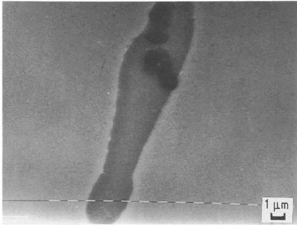
Figure 14 SEM micrograph showing no inclusion–matrix decohesion. Material 3, same specimen as Fig. 13. After hydrogen damage test. Observed zone * in Fig. 2.
